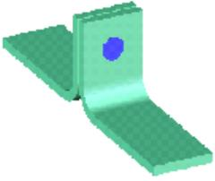
This JSAM8 tool calculates the Failure strength of the riveted T-peel joint.
