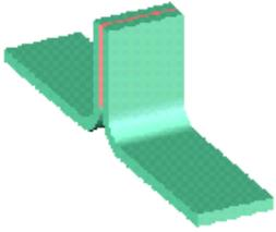
This JSAM10 tool calculates the strength of the adhesively bonded T-peel joint.
