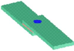
This JSAM7 tool calculates the strength of the combined Rivet/bond lap joint and displays its probable failure mode. The combined failure strength is determined using a mathematical approach that combines the ultimate failure strengths of the rivet joint with the Volkersen Elastic strength of the adhesive.
