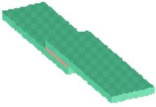
This JSAM5 application calculates the Volkersen elastic failure strength of the adhesively bonded lap joint. This Jsam module is applicable to equal thickness adherends only. Offering a simpler input table.
