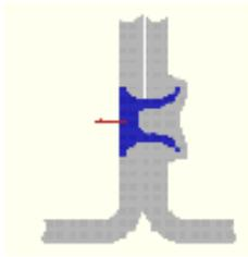
This JSAM9 tool calculates the axial Load in the rivet of the riveted T-peel joint at joint failure.
