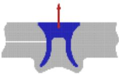
The JSAM4, calculates the equivalent self-piercing rivet diameter ( ESRD) that would be used in place of a weld diameter, in the ACM2/NASTRAN program.
