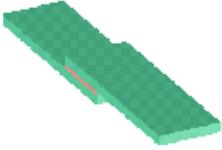
This JSAM6 application calculates the Volkersen elastic failure strength of the adhesively bonded lap joint.
