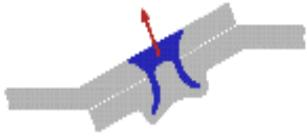
This JSAM3 tool calculates the Load in the rivet of the riveted Lap joint at joint failure.
