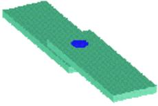
This JSAM2 application calculates the failure load strength of a riveted Lap joint and also displays the Failure mode. Failure modes displayed include;
